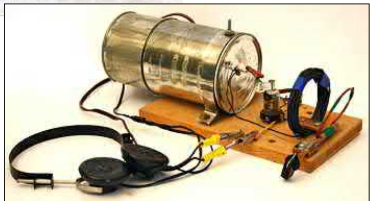
Replicas of the 'Tin can' radio were built by Werner Bösterling (left) and Hans Necker of the 'Internationales Radiomuseum Hans Necker' (below) where it is currently on display.
