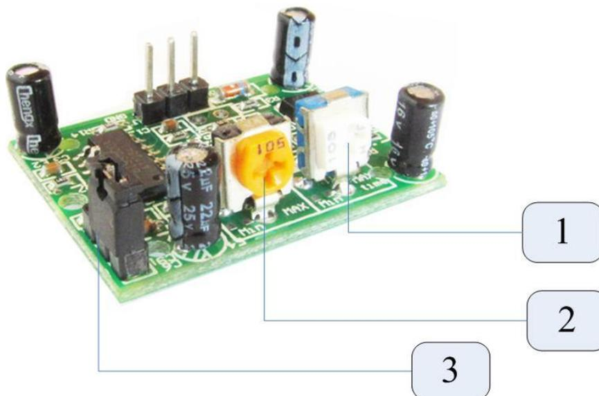
(1) Delay Time Potentiometer; (2) Distance Potentiometer; (3) Trigger Mode Jumper
