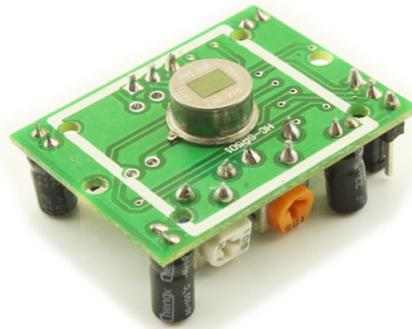
This module is based on BISS0001 PIR motion detector IC, which processes the output of the analog sensor and transforms it in a digital signal. This module allows you to detect motion, and its most frequent use is to determine when a human has moved into the sensing range.
