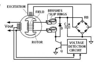
AC is converted to DC by the rectifier bridge "RB"and filter capacitor "C". The detection circuit compares a voltage
