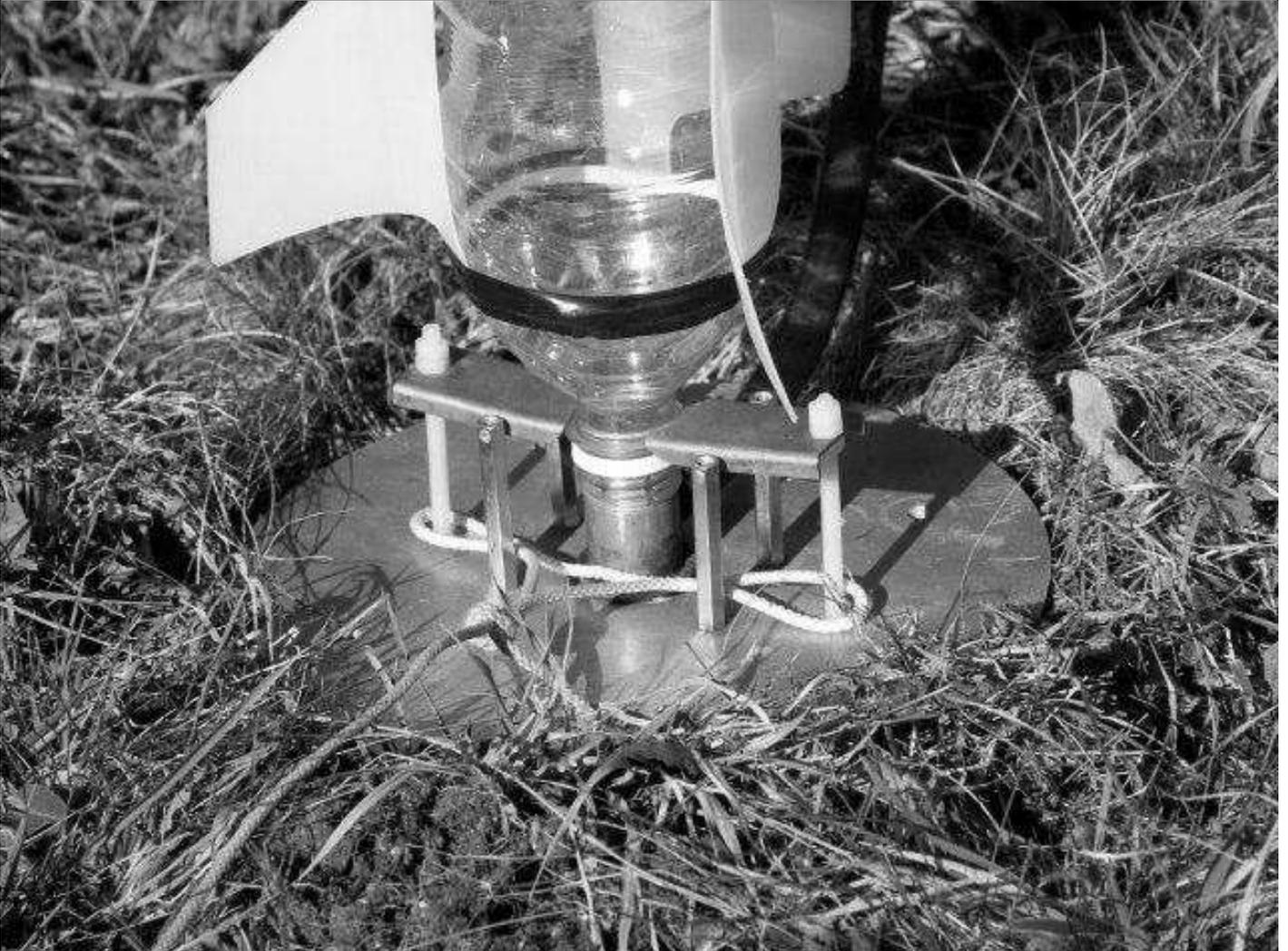
Release cord is looped around the Nylon rods that hold the brass clamps horizontal.
