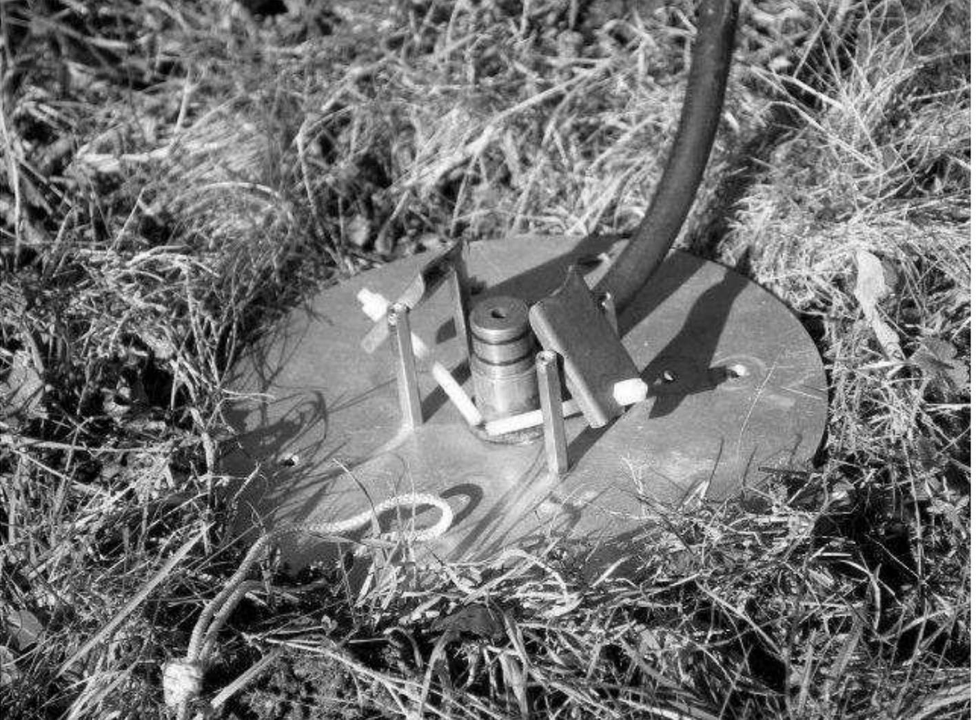
Pulling the release cord bends the Nylon rods in towards the centre of the launcher, opening the clamps.
