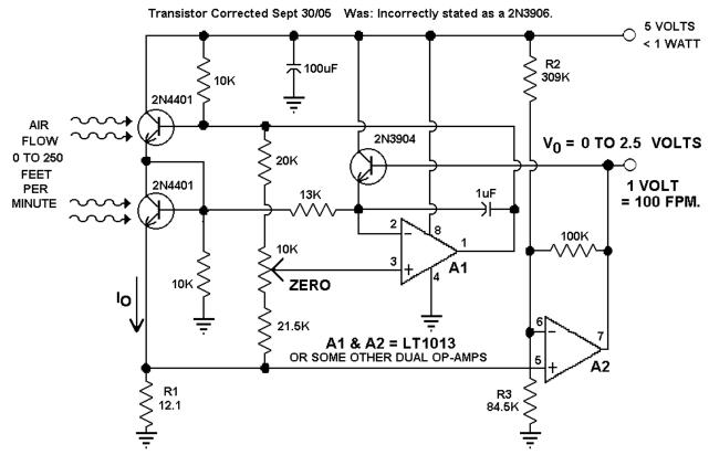
THIS CIRCUIT COMBINES IDEAS FROM TWO EARLIER IFD'S TO IMPLEMENT, LINEARIZED THERMAL ANEMOMETER. AN AMBIENT-TEMPERATURE-COMPENSATED DEVICE, IT IS ROBUST AND POWER EFFICIENT.
