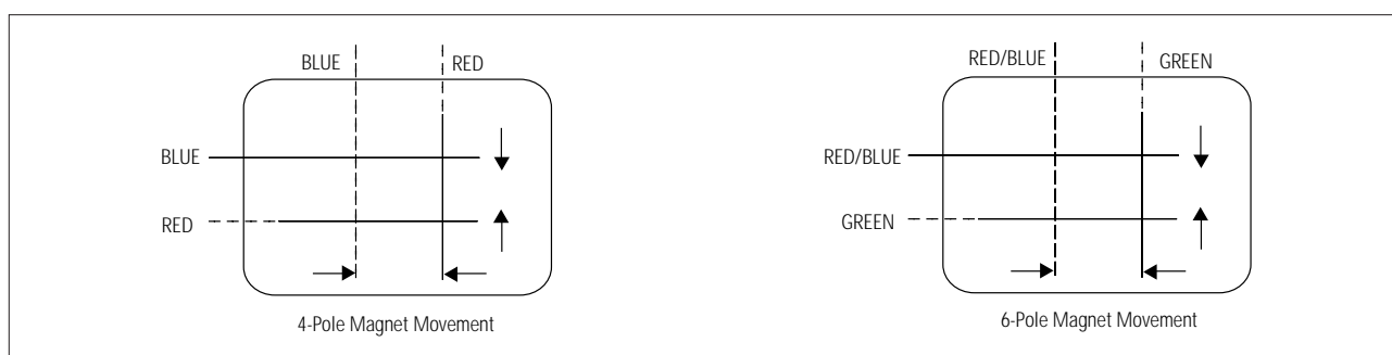
Fig 5-3 Center Convergence Adjustment
