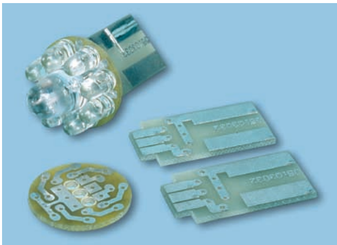
The wedge lamp is made up using the Disc board and two identical Wedge boards. It all goes together as shown in Figs.7 & 8.
