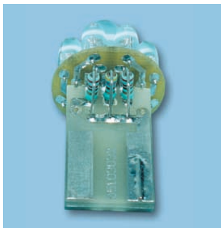
The three current-limiting resistors are mounted vertically on the wedge assembly and can be insulated with heatshrink tubing if desired.
