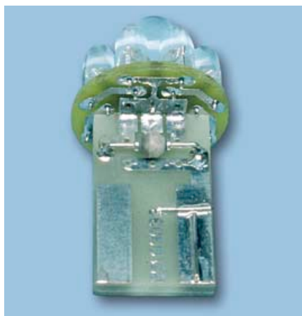
The diode goes on the other side of the wedge assembly. The three long pads on both wedge boards are soldered to matching pads on the disc board.
