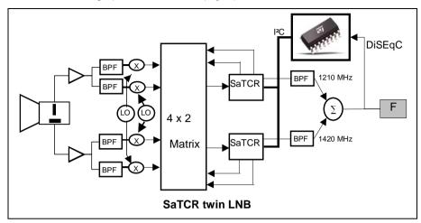
First stage of a SaTCR LNB (up to the matrix) is similar to a conventional LNB. As a consequence, the transponder frequency at the input of a SaTCR device is the same as Ftuner with a classical LNB:
