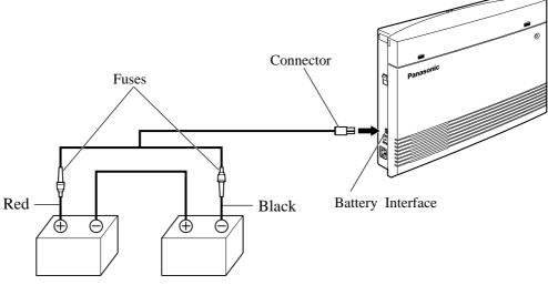
Two Car batteries (12 VDC each)
