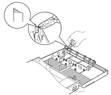
**4.** First, insert the plastic spacer into the hole on the KX-TA30877. Attach the 2 extension connectors to the system, install the KX-TA30877 and secure the 2 extension bolts.
