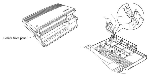
**3.** After cutting the areas, be sure to cut off any excess plastic in order to make the surface smooth.
