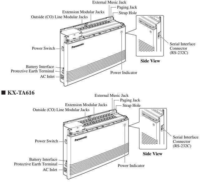
This set is designed for wall mounting only. The wall where the main unit is to be mounted must be able to support the weight of the main unit. If screws other than the ones supplied are used, use screws with the same diameter as the ones enclosed.
